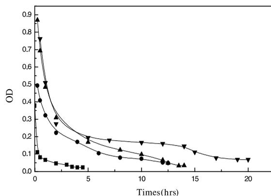
Fig. 5. The sedimentation capabilities of different concentrations of 0.5 CEC-modified montmorillonite in the aqueous solution: 1 g/l (■), 3 g/l (●), 5 g/l (▲) and 7 g/l (▼).
