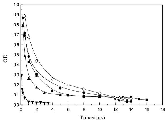
Fig. 2. The sedimentation capabilities of modified montmorillonites: 0.3 CEC (■), 0.5 CEC (●), 0.7 CEC (▲), 1.0 CEC (▼) and natural (◇).
