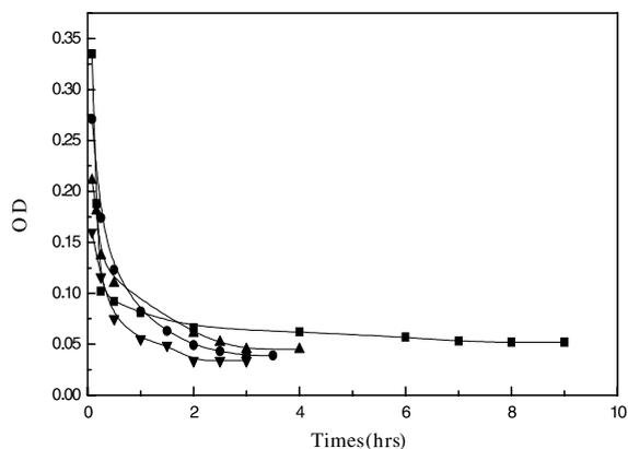
Fig. 7. The sedimentation capabilities of 0.5 CEC-modified montmorillonites sorbed different contents of organic substances: 23.53 mg/g (■), 39.15 mg/g (●), 48.18 mg/g (▲) and 52.95 mg/g (▼).
