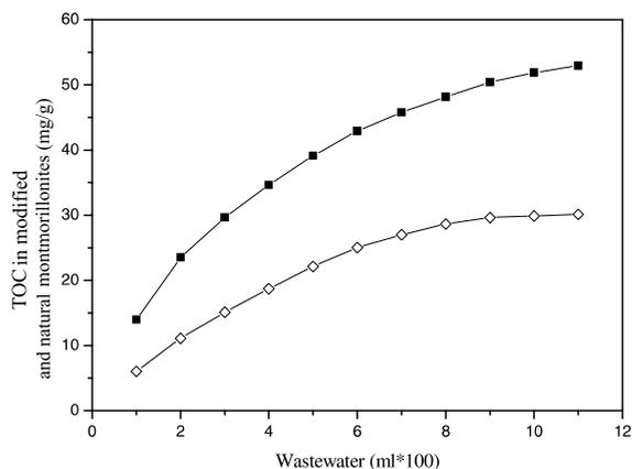
Fig. 6. The relationship of content of organic substances sorbed by modified and natural montmorillonites with the volume of oily wastewater: 0.5 CEC (■) and natural (◇).
