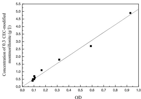
Fig. 1. The relationship of OD with concentration of 0.3 CEC-modified montmorillonite in suspension.
