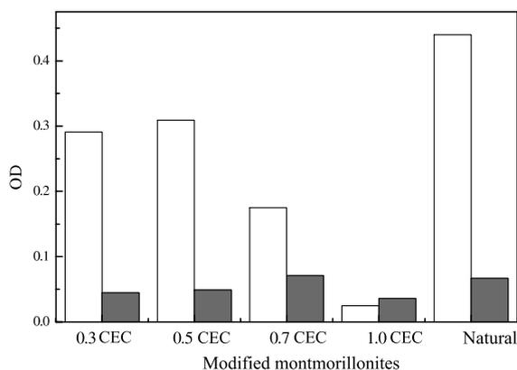
Fig. 4. The comparison between sedimentation capabilities of modified montmorillonites sorbed organic substances and that not sorbed organic substances after 2 h: without sorbed organic substance (□) and with sorbed organic substance (■).
