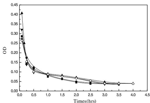
Fig. 3. The sedimentation capabilities of modified montmorillonites sorbed organic substances: 0.3 CEC (■), 0.5 CEC (●), 0.7CEC (▲), 1.0 CEC (▼) and natural (◇).
