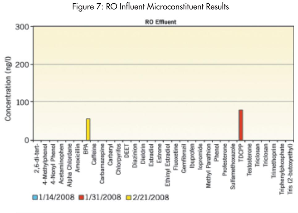
Figure 8: RO Effluent Microconstituent Results
