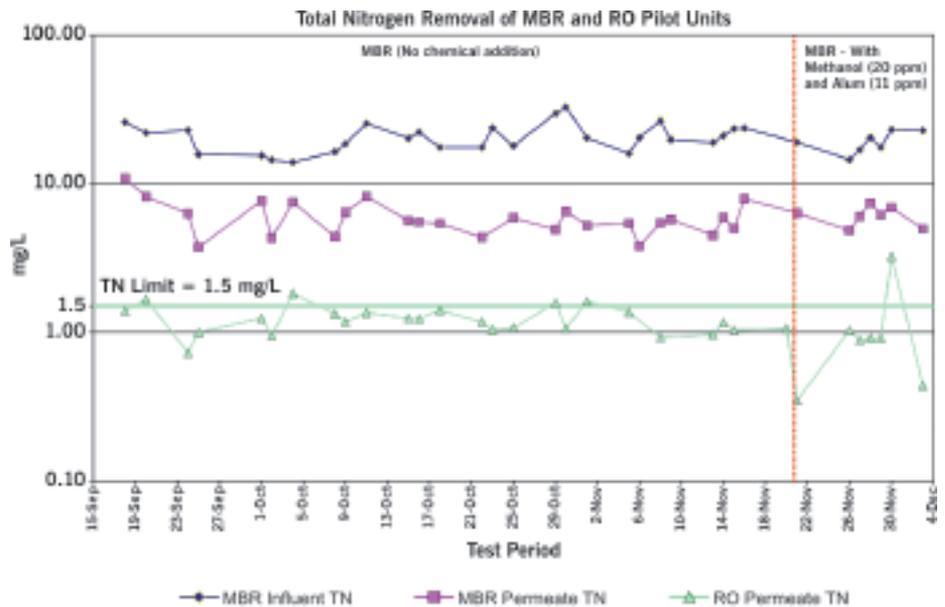
Figure 3: MBR Scheme Total Nitrogen Removal
